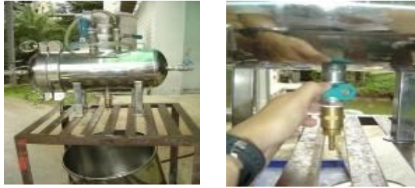
Figure 9. Put receptacle under pressurized tank (left), open valve under pressurized tank (right)
