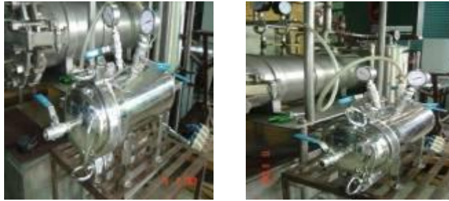
Figure 3. Close a cover of pressurized tank (left), The pressurized tank connected with vacuum (right).
