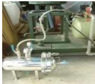
Figure 7. The pressurized tank connected with pump.
